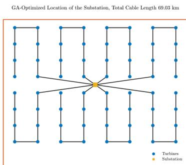
Fig. 4. Optimal substation location with GA algorithm
