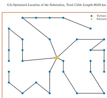
Fig. 7. Optimal substation location with GA algorithm
