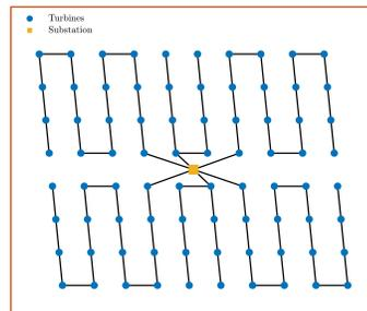
Fig. 11. Optimal substation location with GA
