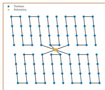
Fig. 12. Optimal substation location with PSO
