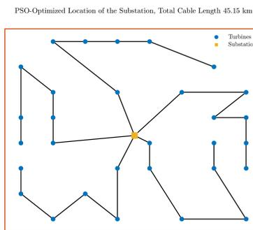
Fig. 8. Optimal substation location with PSO algorithm
