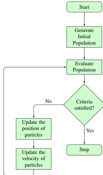
Fig. 2. Flowchart of the Particle Swarm Optimization Algorithm
