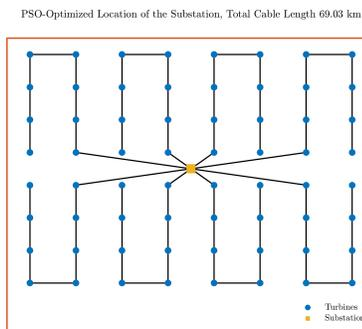
Fig. 5. Optimal substation location with PSO algorithm
